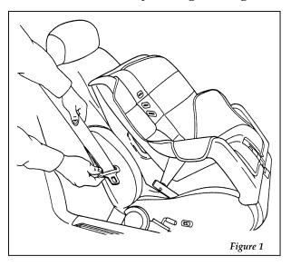
3. While holding the shoulder and lap belt portions together, route the tongue through the child seat according to the child seat manufacturer's instructions. See Figure 2. Be sure that the belt webbing is not twisted.
