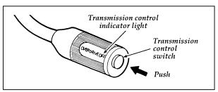
Transmission Control Switch and indicator light (located on the gearshift lever)
