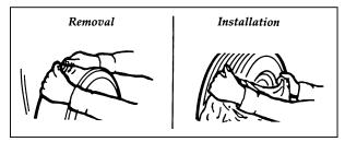
Removal and installation of spare tire cover
