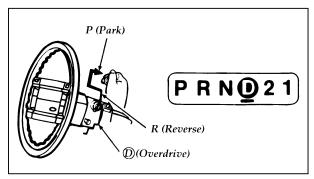
The positions of the column-mounted gearshift
