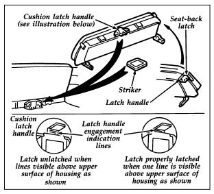
Assembly for installing and removing the rear seat
