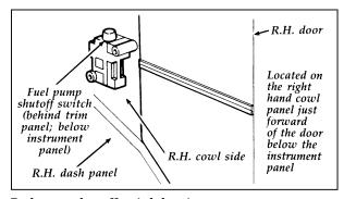
Fuel pump shut-off switch location
