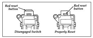
Reset button for fuel pump shut-off switch
