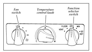
To turn your Heater system on, select any position except OFF. This will turn the fan ON and allow air flow into the vehicle. Select OFF to turn your Heater off. This will turn the fan off and stop outside air from coming into the vehicle.
