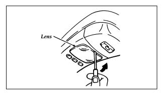
To remove the bulbs, use a screwdriver or coin to push up and rotate counterclockwise  $90^{\circ}$ . The bulb and bulb holder will then drop out from the lamp as shown:
