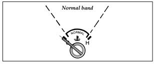
Engine coolant temperature gauge
