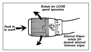
Interval wiper on turn signal lever
