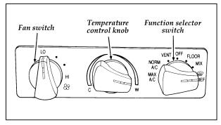
Climate control knobs (Heater A/C system)
