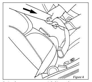
Setting the retractor to automatic locking mode
