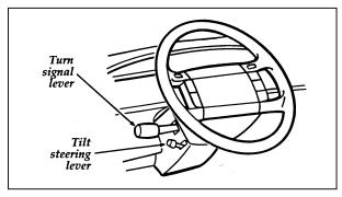
Turn signal and tilt release wheel lever
