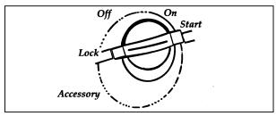
The positions of the key in the ignition lock cylinder.
