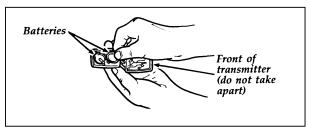
Replacing the batteries
